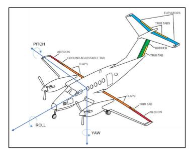
Mr Nishizawa gave evidence that the rudder trim tab was about 1 meter top to bottom and that if it was in full left or right position, it would be a relatively large deflection angle for this kind of aircraft, would be about 3 inches off the centre instead of sitting neutrally aligned to the rudder, and if you were to walk around the aircraft with the trim tab in full deflection, it would be obvious.
